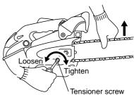
Tighten the nuts securely with the bar tip held up (11.8-14.7 N.m./120-150 kg-cm). Then check the chain for smooth rotation and proper tension while moving it by hand. If necessary, readjust with the chain cover loose.
